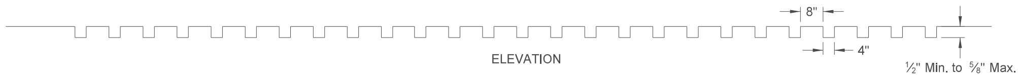
SAW SLOTTED RUMBLE STRIP DETAIL
