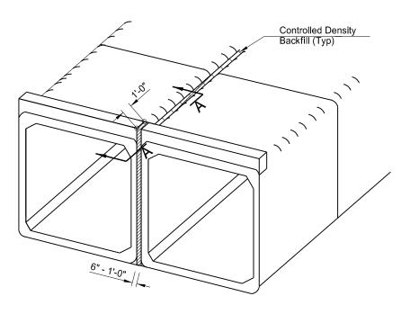
**MULTIPLE CELL INSTALLATION** (Wings & Apron Not Shown)
