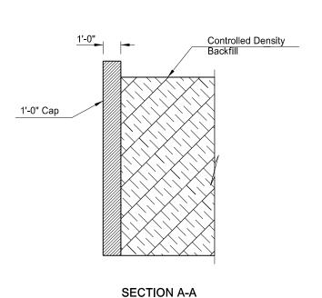
The intent of this drawing is to show only the placement of the controlled density backfill between adjacent barrels. The representation of the number of barrels is arbitrary.
