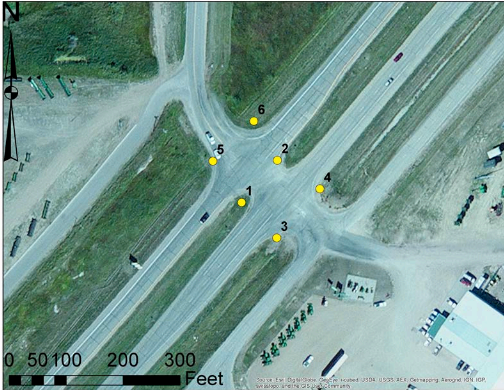
Figure 1 – Existing Intersection and Boring Locations
