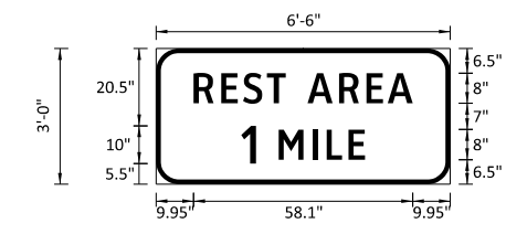
Dimensions are in inches.tenths Letter locations are panel edge to lower left corner PANEL STYLE: ND_Conv_General Services.sst
