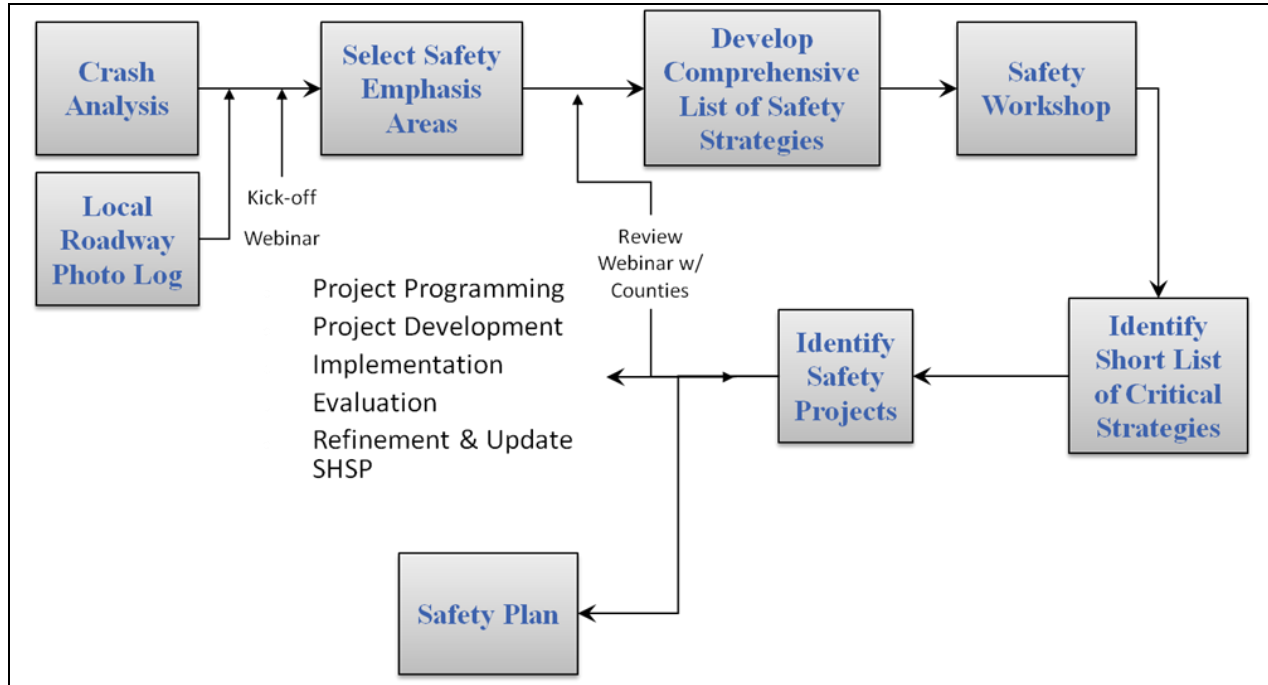
FIGURE 1-3 Local Road Safety Program Safety Plan Approach
