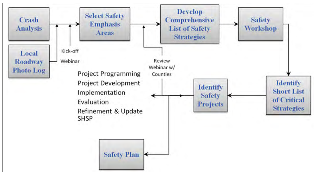
FIGURE 1-3 Local Road Safety Program Safety Plan Approach
